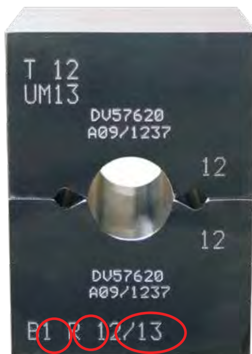
A, Cylindrical Press Dies (one sided rounding)
