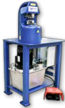
75-ton Swager mounted on a work bench.
