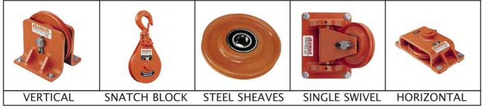
Jeamar steel sheaves are manufactured from the highest quality, fine-grain steel, ensuring uniformity of material, consistent high quality and greater strength. Rope grooves are work hardened during the forming process, which substantially increases the life of the sheave. All sheaves are fitted with lifetime lubricated bearings.
